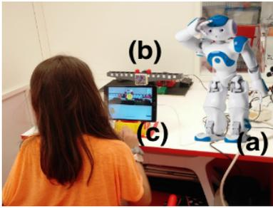
**Figure 1: Example of an interaction.** The robot (a) interacts with a child in the balance beam educational task. The child places various weights on the Smart Balance Beam (b) and predicts where the scale will fall using the easelscope (c). (Image has been edited to represent the new setup.)
